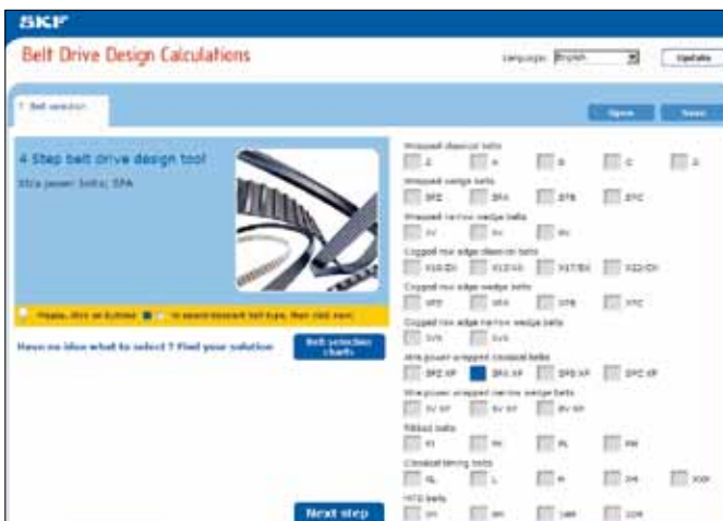
Step 1. Choose your preferred belt type out of a comprehensive list of belt profiles to start the calculation.
